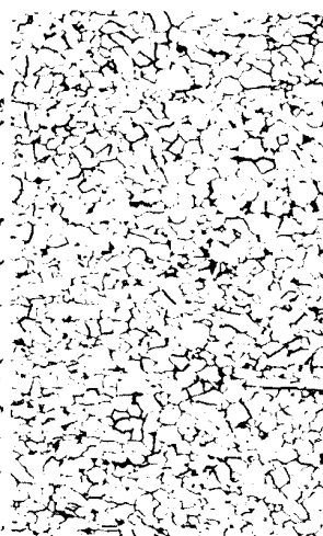
Nital 100× 9 Nominal ASTM grain size No. 9 (specimen has a calculated grain size of 8.97)
