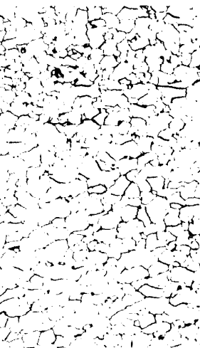
Nital 100× 8 Nominal ASTM grain size No. 8 (specimen has a calculated grain size of 8.03)
