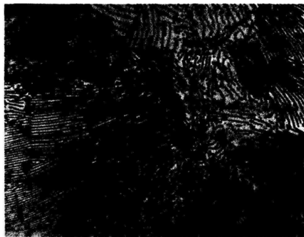
FIGURE 9.8 Microstructure of a slowly cooled eutectoid steel. The microstructure consists of lamellar eutectoid pearlite. The dark etched phase is cementite, and the white phase is ferrite. (Etch: picral; magnification 650 \times .) (United States Steel Corp., as presented in "Metals Handbook," vol. 8, 8th ed., American Society for Metals, 1973, p. 188.)
