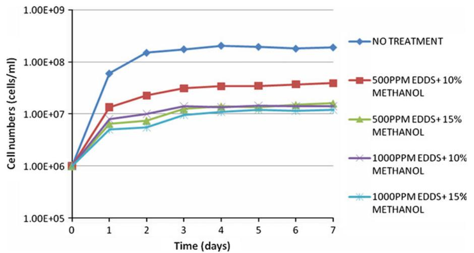
**Fig. 2** Effects of the triple biocide cocktail treatment of EDDS and methanol plus 30 ppm glutaraldehyde on planktonic SRB growth in ATCC 1249 medium
