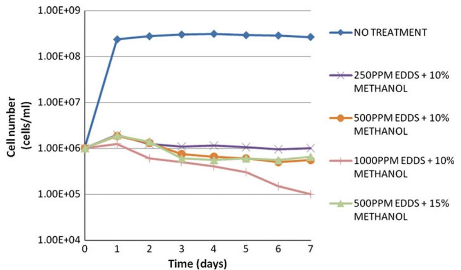
**Fig. 3** Effects of the triple biocide cocktail treatment of EDDS and methanol plus 30 ppm glutaraldehyde on planktonic SRB growth in 1/4 strength diluted medium
