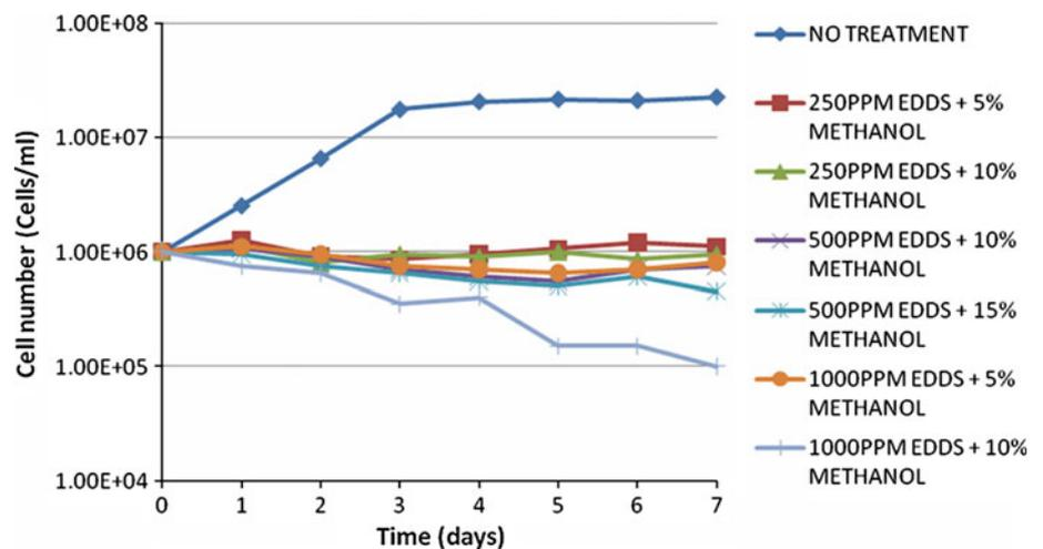
**Fig. 4** Effects of the triple biocide cocktail treatment of EDDS and methanol plus 20 ppm glutaraldehyde on planktonic SRB growth in 1/4 strength diluted medium
