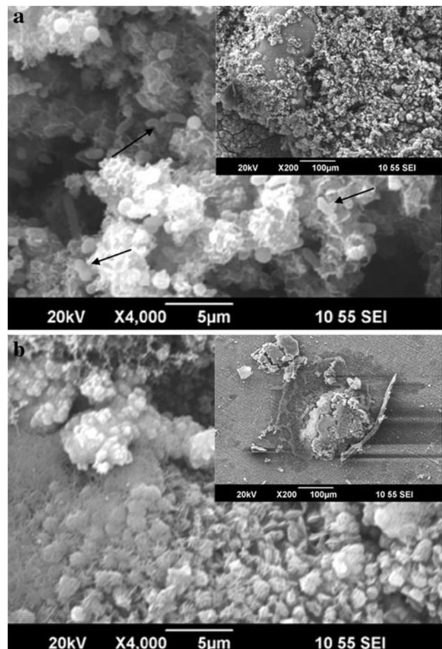
**Fig. 5** Effect of 15% methanol + 50 ppm glutaraldehyde on treating an established SRB biofilm in ATCC 1249 medium with initially 25 ppm  $\text{Fe}^{2+}$  after 9 days of exposure. **a** Combined with 0 ppm EDDS, sessile SRB are visible. *Arrows* indicate SRB cells; **b** combined with 1,000 ppm EDDS, sessile SRB are hard to find
