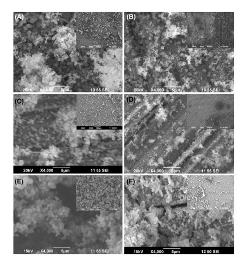
Fig. 4 SEM images for coupons in ATCC 1249 medium covered with well-established biofilms for 7 days then they were treated with a 30 ppm THPS + 500 ppm EDDS + 6.6 ppb p-amino acid mixture, b 30 ppm THPS + 500 ppm EDDS + 6.6 ppm p-amino acid mixture. Scale bars for the small inserted images are 100 μm
