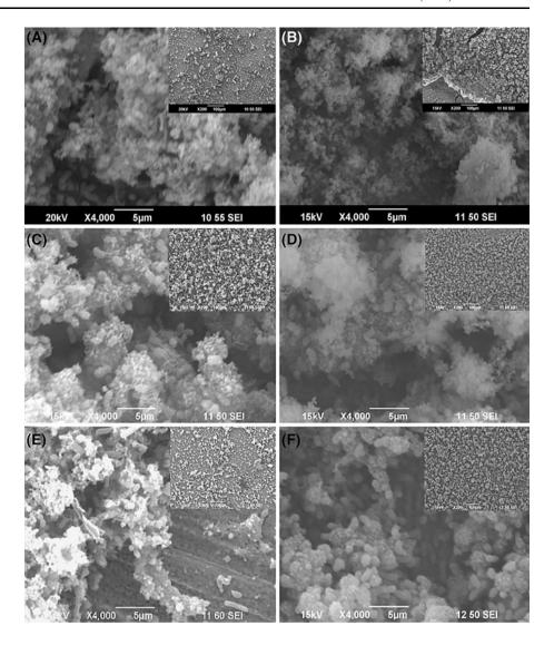
Fig. 2 SEM images for 7-day coupons in ATCC 1249 medium with a 30 ppm
