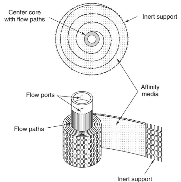
**Figure 4.** Structure of a Zetafinity cartridge.
