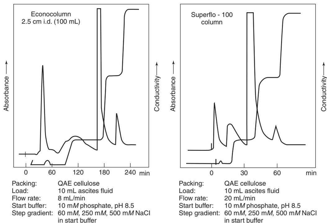
**Figure 10.** Comparison of AFC and RFC columns. (Courtesy of Sepragen Corp.)
