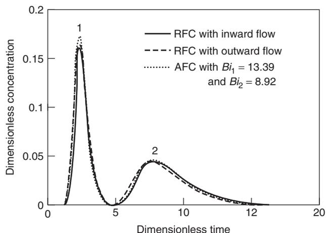
**Figure 17.** Simulated comparison for inward and outward flow RFC and AFC.
