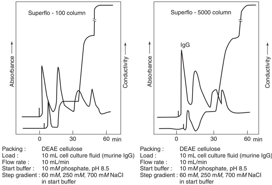
**Figure 19.** A 50-fold scale-up example using Superflo columns.
