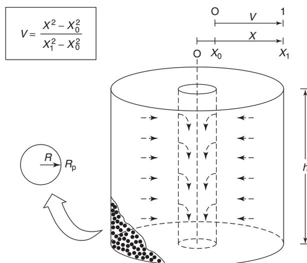
**Figure 16.** Anatomy of an inward flow RFC column.
