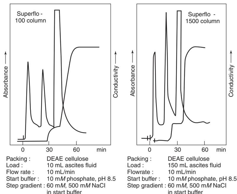
**Figure 18.** A 15-fold scale-up example using Superflo columns.
