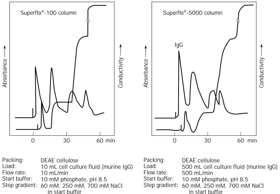
**Figure 16.** A 15-fold scale-up example using Superflo® columns.
