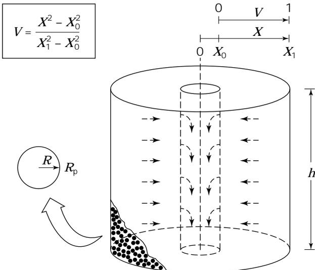
**Figure 13.** Anatomy of an inward-flow RFC column.
