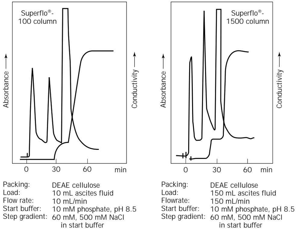
**Figure 15.** A 15-fold scale-up example using Superflo® columns.
